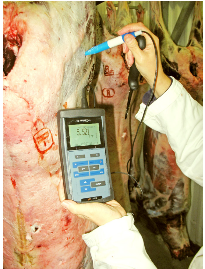
Figure 5. Meat pH measured 24 hours after slaughter is a predictor of meat quality. A value of 5.5 to 5.7 is within the normal range (source: B. Åhman).
